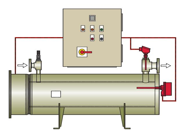
Midcom design and manufacture a wide range of Electric Control Panels for their range of Electric Heaters, Pumping systems and Packaged equipment. In particular their Heaters range from 1kW through to 2000kW and the appropriate Control Panels and Integrated systems can be supplied. The operation of the Electric Heater is only as good as the system that controls it. Matched panels supplied by Midland Combustion are correctly designed to ensure accurate temperature control.
